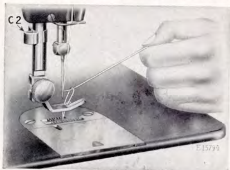
FIG. 12. DRAWING UP THE BOBBIN THREAD
