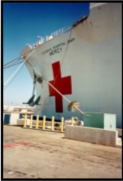
Fig. 2-30. Placement of rat guards.
